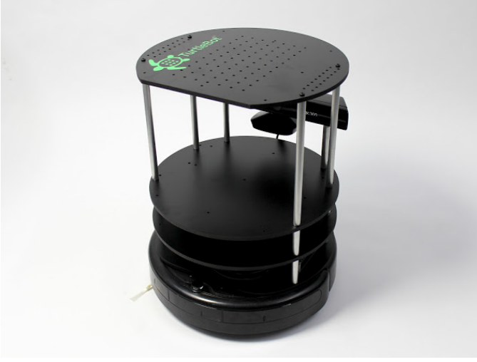
Fig. 1. Turtlebot platform developed by Willowgarage Robotics as an Open Development Platform [9]
