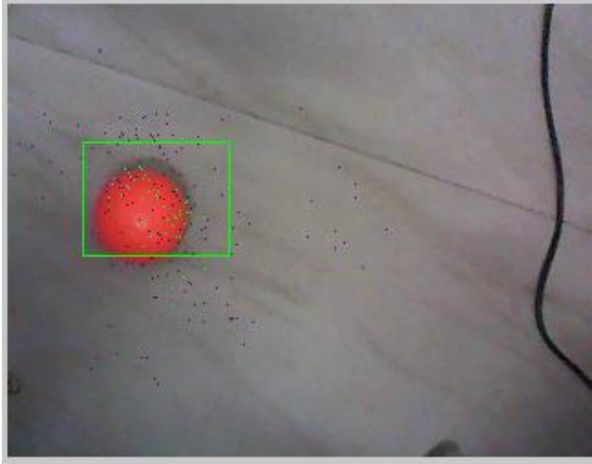
Fig 6.2: Object tracked by the Particle Filter
